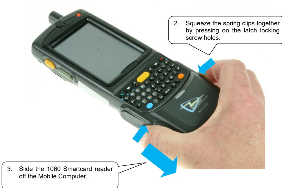
**Figure 3: Detaching from an MC70/75/75A**
