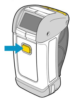
2) Slide the battery cover down and lift it off.
