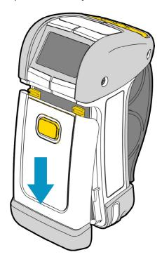
The battery can then be lifted out and replaced. Refit the cover by sliding it back up until the button clicks in place.
