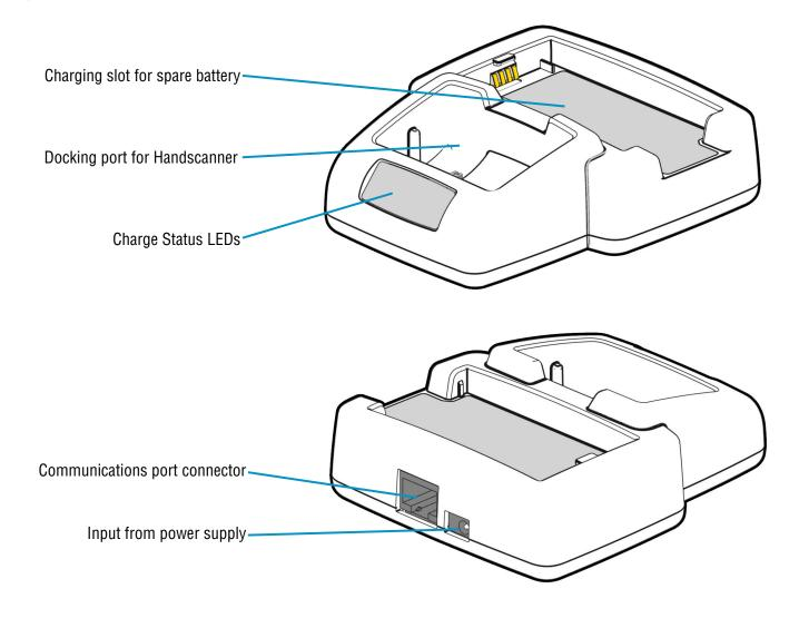
The Charge Status LEDs indicate the state of the spare battery. The spare battery charge feature is independent of the charging of the battery inside the Handscanner.
