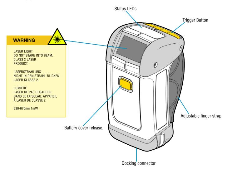
The status LEDs on the top of the Handscanner provide an indication of the operating status of the unit.
