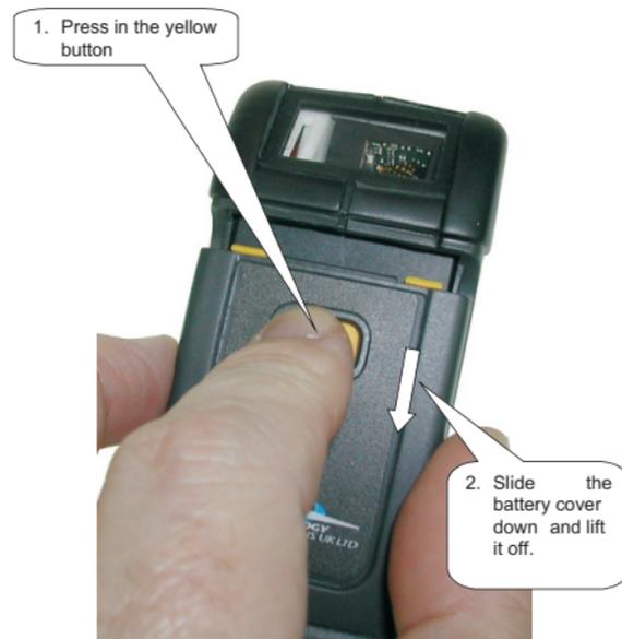
The battery can then be lifted out and replaced. Refit the cover by sliding it back up until the button clicks in place.
