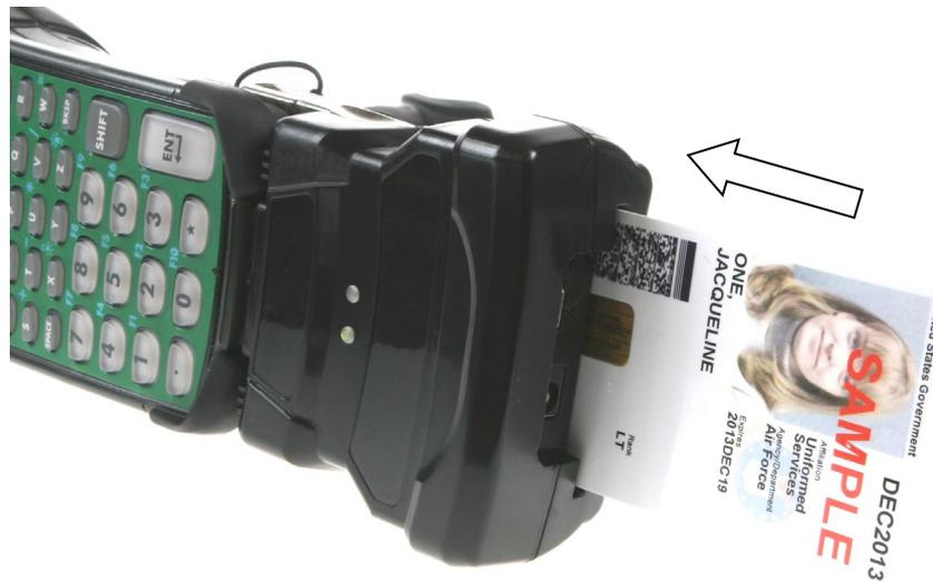
**Figure 6: Inserting a Smartcard**
