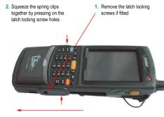
3. Slide the RFID 1059 off the MC70/75
