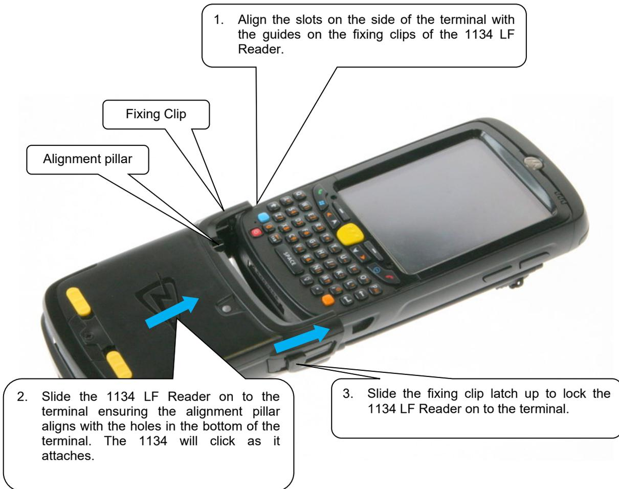
**Figure 2: Attaching to an MC55/65**
