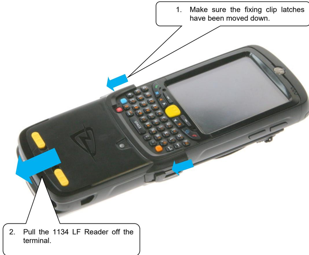
**Figure 3: Detaching from an MC55/65**
