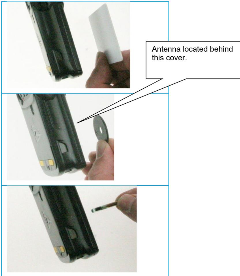
**Figure 4: Antenna location and read direction**
