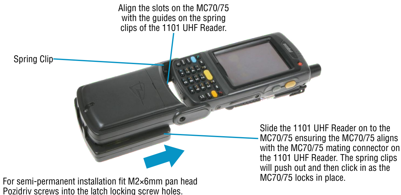
FIGURE 2: Attaching to an MC70/75
