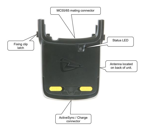
Figure 1: Parts of the 1134 LF Reader
