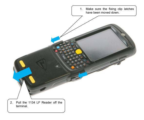
Figure 3: Detaching from an MC55/65
