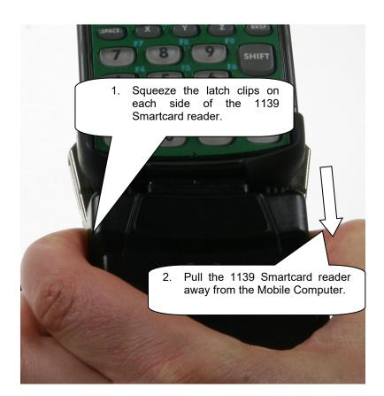
Figure 3: Detaching from a Mobile Computer
