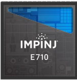
E710 Read rates of \geq 1200 tags/s Up to -88 dBm receive sensitivity
