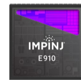
E910 Read rates of \geq 1200 tags/s Up to -92 dBm receive sensitivity
